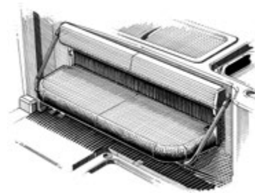
Folding aft bench seat. Patent No. 6,789,494
